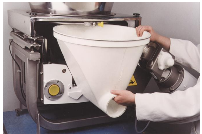
This externally agitated screw feeder has a flexible hopper that's easy to remove and replace for frequent material changeovers.
